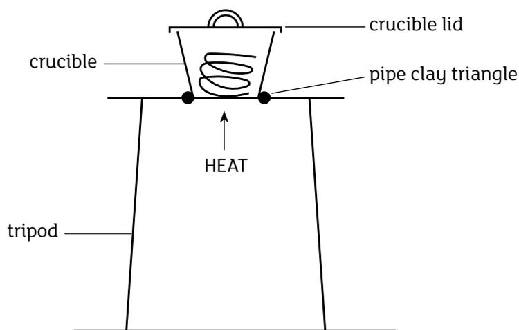
4. Heat the crucible gently to start. Once the crucible is hot, gently lift the lid with the tongs for a few seconds to allow some air to get in.
