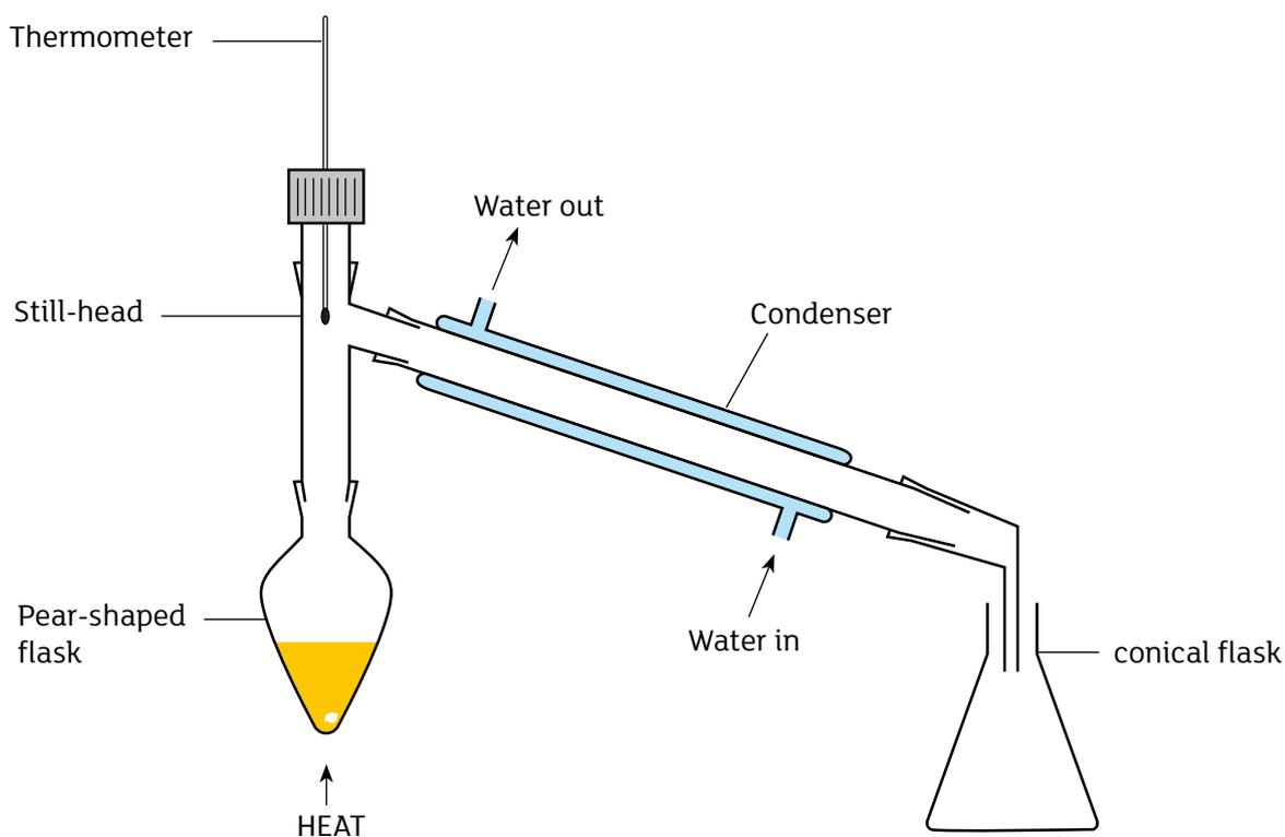
5. Heat the bottom of the pear-shaped flask gently, until  $2\text{--}3\text{ cm}^3$  of liquid has distilled over. Note the temperature that the distillate comes over at.
