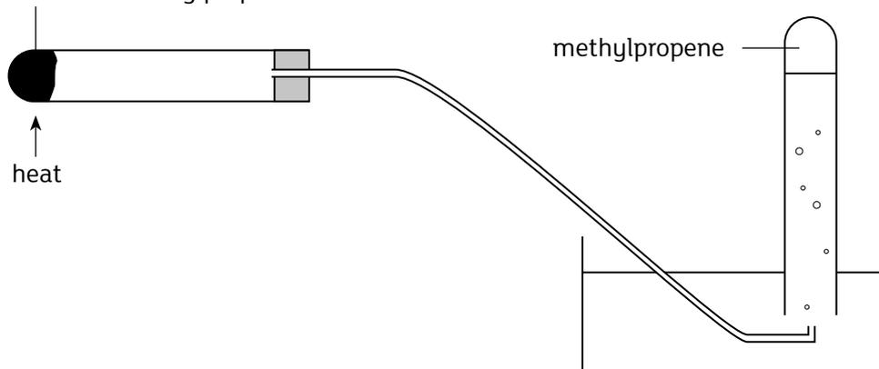
5. Heat the contents of the boiling tube gently and collect the gas produced in the test tube.
