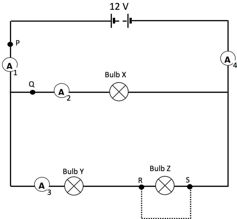
You only have one ammeter so you will need to disconnect the ammeter from position 1 and reconnect it into position 2, then 3, then 4 and record the readings below.
