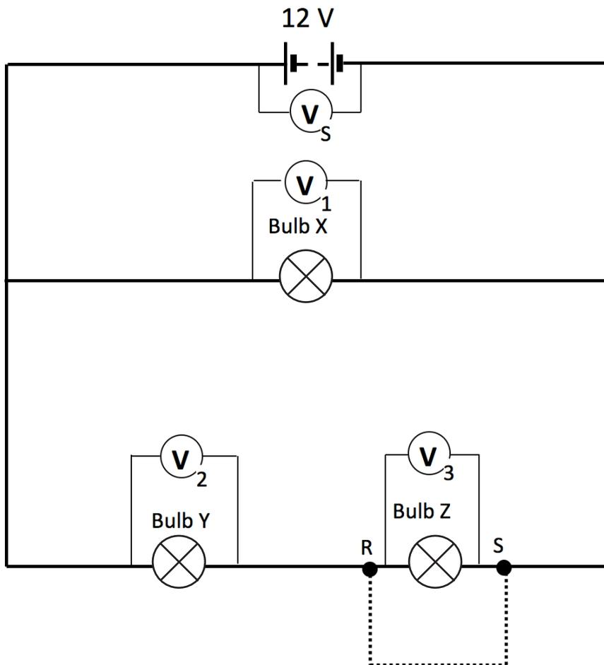
Once again, connect the circuit as shown. Move your one voltmeter around the circuit to the different positions. Do not yet add the wire between R and S.
