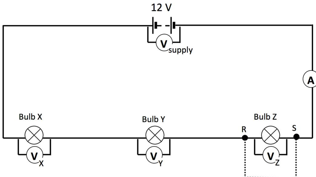
Connect the circuit as shown (ignoring the dotted wire) with the ammeter as labelled and your one voltmeter positioned across the supply as shown. Then move the voltmeter to each of the positions X, Y and Z as shown and record your results.
