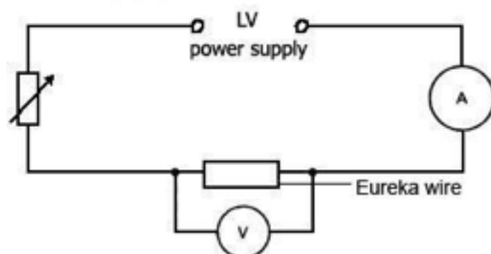
3. Calculate the ratio of p.d./current for each pair of values. Record in the table.
