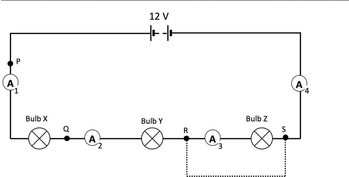
You only have one ammeter so you will need to disconnect the ammeter from position 1 and reconnect it into position 2, then 3, then 4 and record the readings below.
