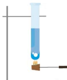
Hold the burning food under the test tube of water. *STEP 8*
