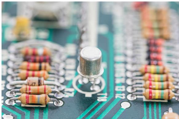
Electronic circuits are usually constructed on Printed Circuit Boards (PCBs). These not only hold the components in place but make the electrical connections to connect the components together. PCBs consist of a layer of copper, which is a very good conductor of electricity, glued to an insulating board. Areas of copper may be removed to leave copper pads for the components to be soldered to, and copper tracks to join the copper pads.
