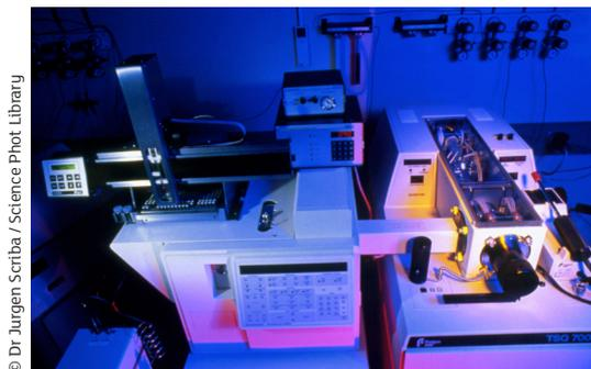
A gas chromatography machine (left) connected to a mass spectrometer (right) in a forensic laboratory. This equipment is sensitive enough to detect minute quantities of illegal drugs in the hair of a suspect - weeks after any drugs were taken.
