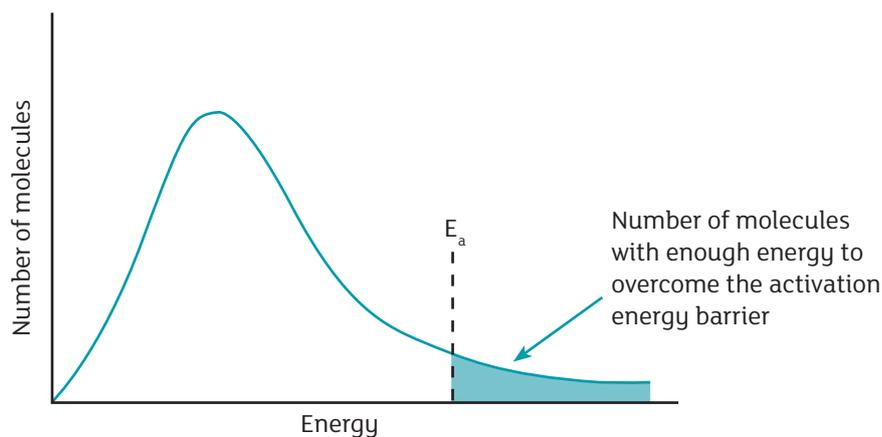
Maxwell-Boltzmann distribution showing the activation energy for the uncatalysed reaction ( $E_a$ ).
