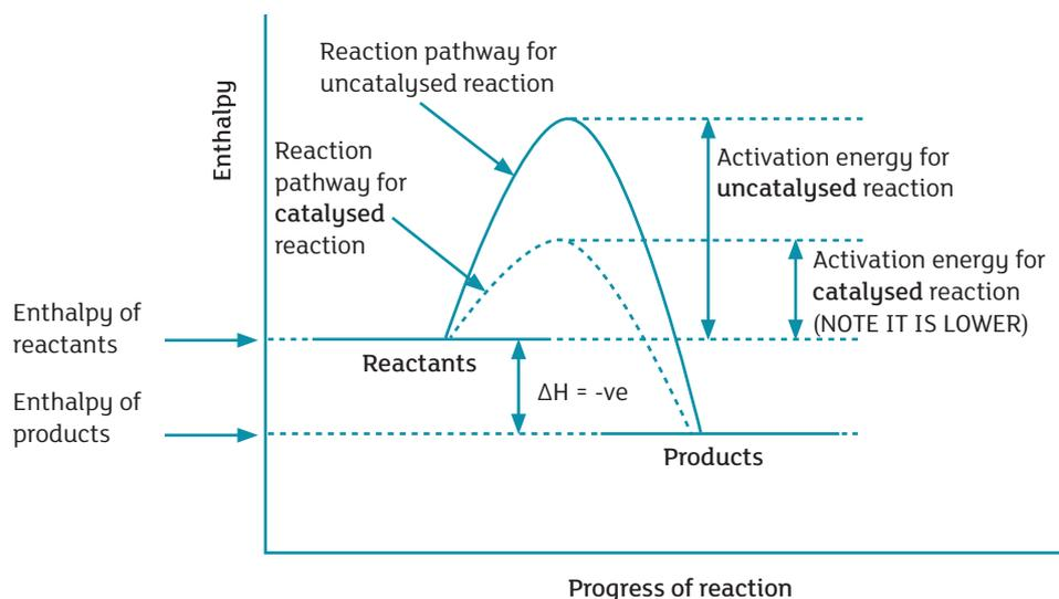
Enthalpy level diagram for an exothermic reaction
