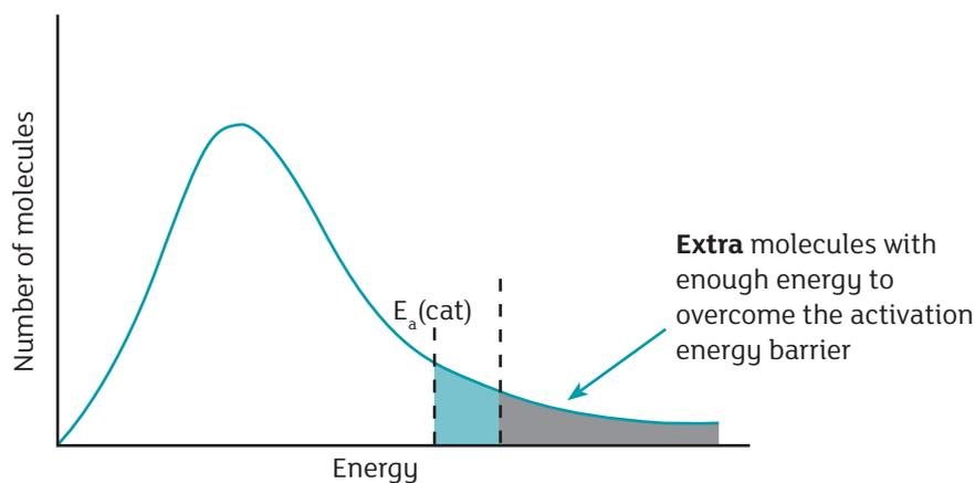
Maxwell-Boltzmann distribution showing the activation energy for the catalysed reaction,  $E_a$  (cat).
