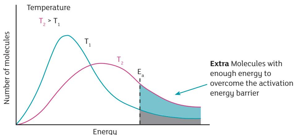
If a catalyst is used, the position of the activation energy on the curve shifts to the left which results in more gas particles having energy greater than or equal to the activation energy, leading to a faster reaction rate.
