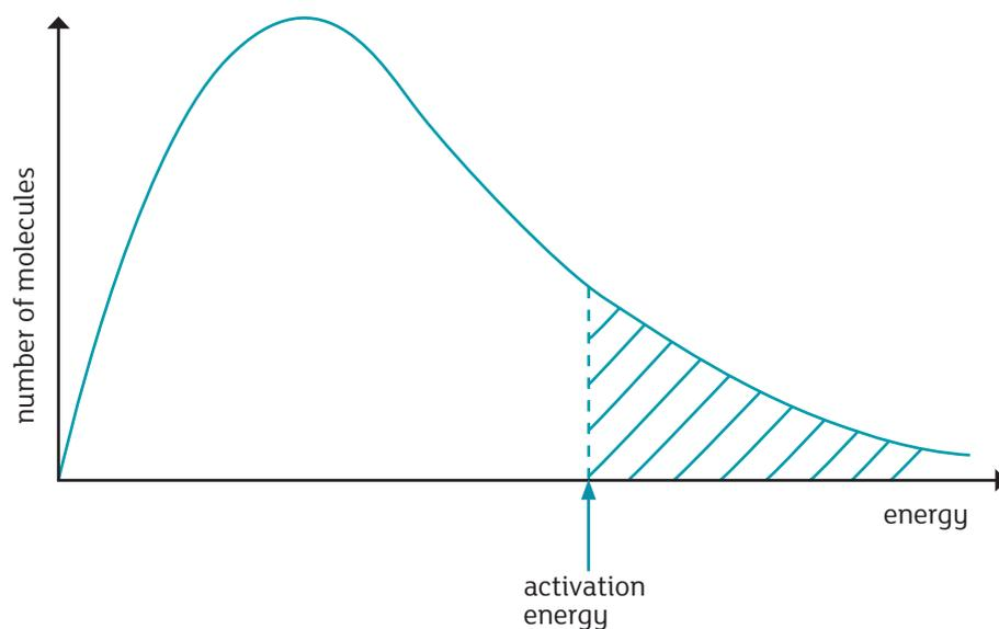
The area under the curve is a measure of the total number of particles present. For a reaction to happen, particles must collide with energies equal to or greater than the activation energy for the reaction. Notice that the large majority of the particles don't have enough energy to react when they collide.
