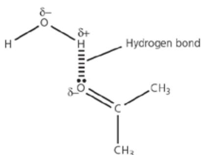
Hydrogen bonds between water and propanone molecules
