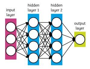
Each connection in the neural network is weighted and algorithms are used to calculate the weighted sum of any inputs into a node in order to generate an output value. A neural network does not have to be programed to learn explicitly; it learns by itself, much in the same way a human brain would learn.
